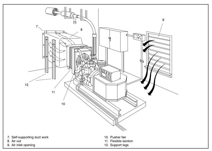
Figure 4-8 Radiator-Cooled Generator Set Installation
